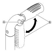
1. Fully depress button (A) and fold up respectively fold down the push handle (B) until it audibly engages.
